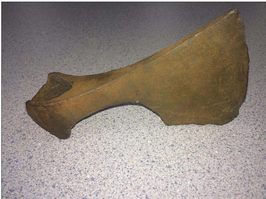
**Fig. 1.** 3D-printed Viking Age axe head. 3D-printed with composite iron filament and post-processed with salt and vinegar to create a rusted finish. Viking axe 3D scan is by Snorri and is licensed under Creative Commons-Attribution license <http://www.thingiverse.com/thing:1609633>. Photograph and print by Jennifer Grayburn
