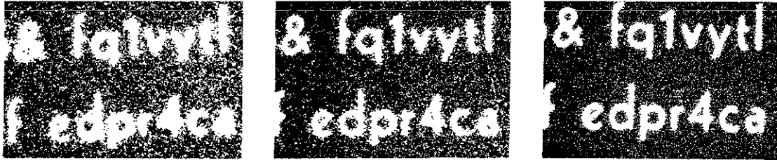
Figure 3. Reproduction of a photo-micrograph illustrating Classic QIs at marginal (3.6), medium (5.0), and high (8.0) levels. 6
