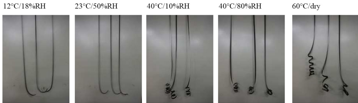
Fig. 6: Macroscale physical deformations observed in tape ends after aging
